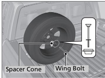
3. Place the spacer cone onto the wheel hub, then secure the flat tire to the pickup bed with the wing bolt as shown.
