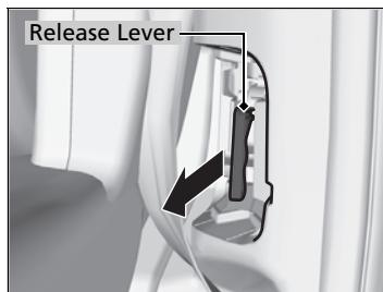
3. Pull the release lever as shown.
