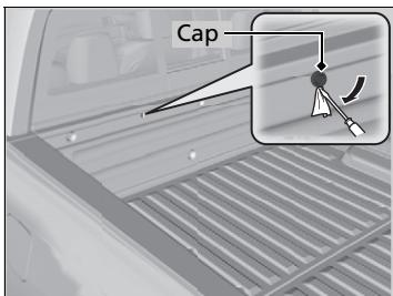
2. Wrap a cloth around the tip of a small flat-tip screwdriver. Put it into the cap as shown in the image, and remove the cap.
