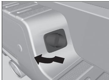
1. Remove the license plate light assembly by pulling it towards you, and then pulling the front edge upward.
