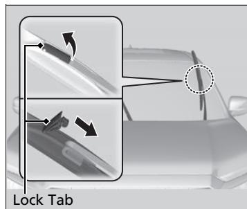
2. Using a flat-tip screwdriver, pry up on the edge of the lock tab to release it.
