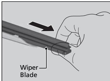
4. Slide the wiper blade out of the holder by pulling the tabbed end out.
