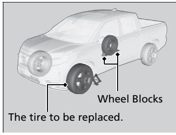
6. Place a wheel block or rock in front and rear of the wheel diagonal to the flat tire.
