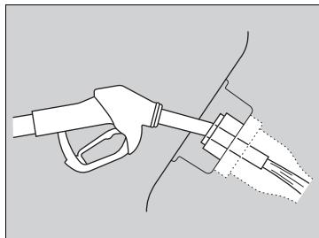
4. Place the end of the filler nozzle on the lower part of filler opening, then insert it slowly and fully.
