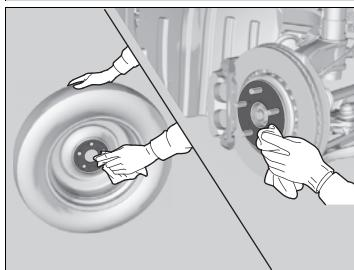
2. Wipe the mounting surfaces of the wheel with a clean cloth.
