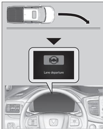
The front camera behind the rearview mirror monitors left and right lane markings (in white or yellow). If your vehicle is getting too close to detected lane markings without a turn signal activated, the system, in addition to a visual alert, applies steering torque and alerts you with rapid vibrations on the steering wheel, to help you remain within the detected lane.
