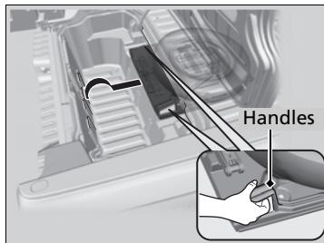
3. Pull out the tire tray with the handles, and hook the rear of the tire tray to the guides on the back edge of the trunk.
