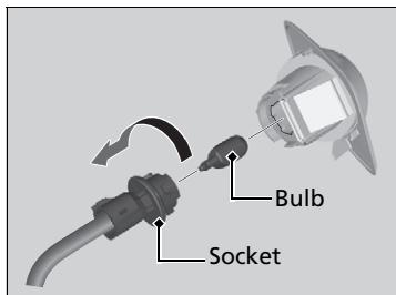
2. Turn the socket counter-clockwise and remove it. Remove the old bulb.
