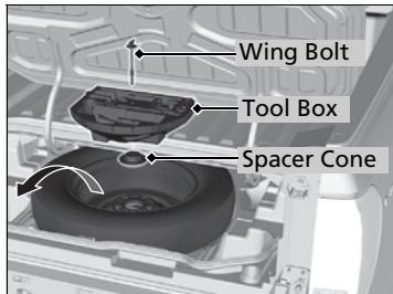
5. Unscrew the wing bolt, and remove the tool box and the spacer cone. Then, remove the compact spare tire.
