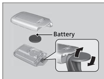
» Replacing the Remote Battery
