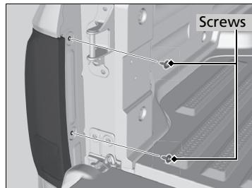
1. Use a phillips-head screwdriver to remove the screws.
