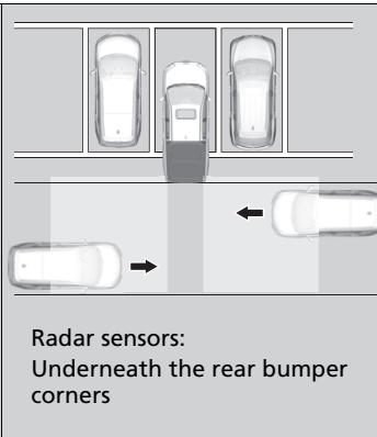
When a vehicle is detected approaching from a rear corner, Cross Traffic Monitor alerts you with a buzzer and a displayed warning.
