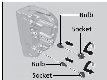
3. Turn the socket counter-clockwise and remove it. Remove the old bulb.
