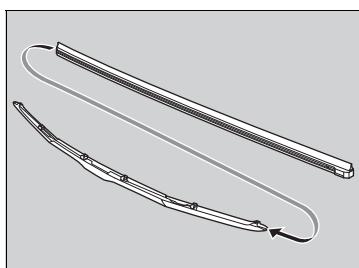
6. Slide the new wiper blade onto the holder from the bottom end.
