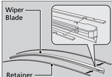
5. Remove the retainers from the wiper blade that has been removed, and mount to a new wiper blade.
