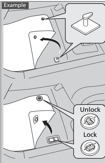
The driver's floor mat hooks over floor anchors, which keep the mat from sliding forward.
