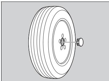
1. Remove the center cap and place the tire on the pickup bed.
