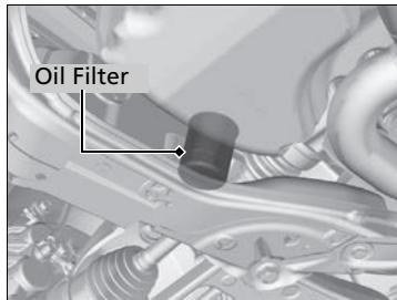
6. Remove the oil filter and dispose of the remaining oil.
