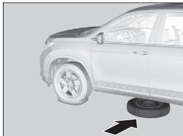
7. Place the compact spare tire (wheel side up) under the vehicle body, near the tire that needs to be replaced.
