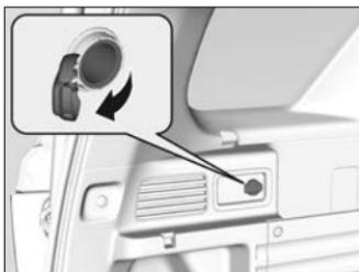
**!** Do not insert an automotive-type cigarette lighter element. This can overheat the accessory power socket.
