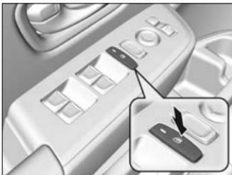
When the power window lock button is set to ON (indicator on), any window other than that on the driver's side will not operate.
