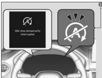
The Auto Idle Stop suspend indicator (1) comes on and a message appears on the driver information interface when the Auto Idle Stop system cannot be activated.
