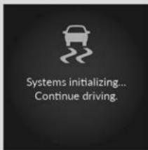
After re-connecting the 12-volt battery: if various indicators come on and the message on the left is displayed on the driver information interface, with the engine running, turn the steering wheel to the left until it stops then to the right until it stops, then drive a short distance at more than 12 mph (20 km/h). If the indicator does not go off, have your vehicle checked by a dealer.
