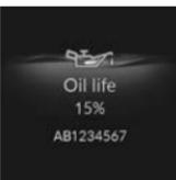
Oil life 15% AB1234567                                                                          | The remaining engine oil life is 15 to 6 percent. Roll the right selector wheel to switch to another display.                                                                                                                                                   |
