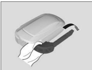
[2] With the buttons facing down, remove the upper half of the cover by carefully prying on the slot with the key grip.
