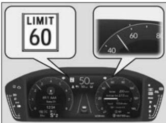
Shows certain detected traffic signs while driving. If speed limit warning is activated, the sign icon blinks when the maximum speed of the traffic sign detected is exceeded by a threshold, when compared with the vehicle speed.
