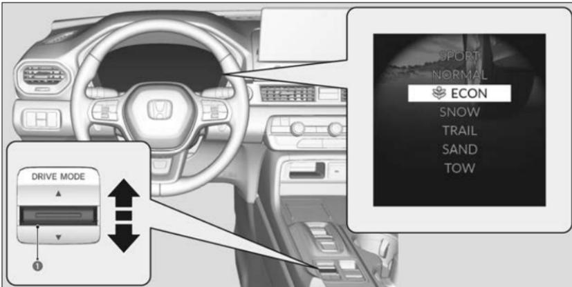
The mode may not be able to be changed under some driving conditions. If there is a vehicle system failure, a message will also appear on the driver information interface, and you cannot change the mode.
