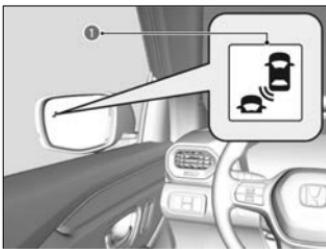
When the system detects a vehicle, the blind spot information system alert indicator (①) on the outside door mirror on both sides comes on in the following situations:
