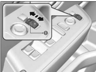
If activated, either side door mirror automatically tilts downward when you put the transmission into **R**: this improves close-in visibility on the selected side of the vehicle when backing up. The mirror automatically returns to its original position when you take the transmission out of **R**.
