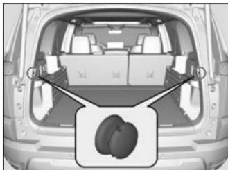
Use the cargo hooks to secure cargo in the cargo area.
