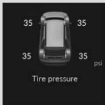
To select the tire pressure monitor, set the power mode to ON, and roll the right selector wheel until you see the tire pressure screen.
