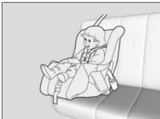
We strongly recommend placing a forward-facing child seat in a rear seating position.
