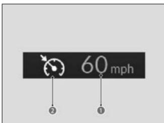
When you turn off cruise control by pressing the **CANCEL** button or depressing the brake pedal, the prior set speed (1) is displayed on the gauge in gray.
