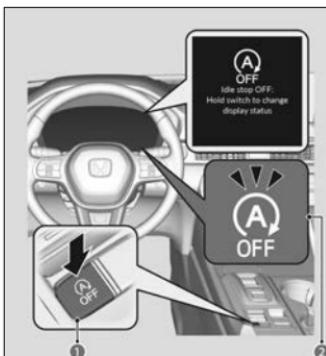
To turn the Auto Idle Stop system off, press Auto Idle Stop **OFF** button (1). The Auto Idle Stop system stops.
