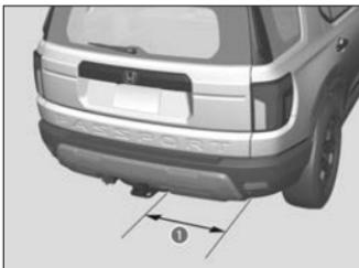
Use a forward and back kicking motion for about 1 second under the passenger side of the rear bumper to open or close the power tailgate while carrying the keyless remote.
