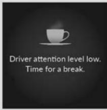
If one bar lights up, the **Driver attention level low. Time for a break.** message will appear, a beep will sound, and the steering wheel will vibrate.
