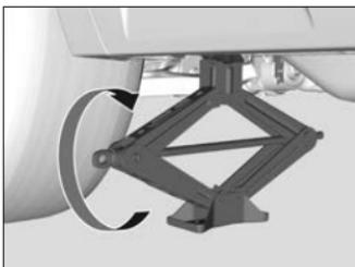
[2] Turn the end bracket clockwise as shown in the image until the top of the jack contacts the jacking point.
