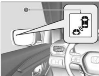
When you operate the turn signal lever in the direction of a detected vehicle, the blind spot information system alert indicator blinks and the beeper sounds.
