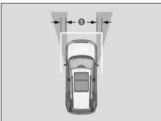
Images of the front side of the vehicle captured by side cameras are displayed on the display. Approximate distance (1) the projection lines indicate is 16 inches (40 cm) from the vehicle.
