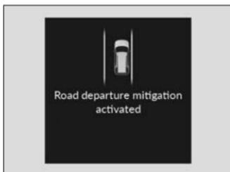
If Lane Keeping Assist System (LKAS) is off, the message may appear if the system has determined that there is a possibility of your vehicle crossing over detected lane markings, the outer edge of the pavement (into a grass or gravel road shoulder) or oncoming vehicle.
