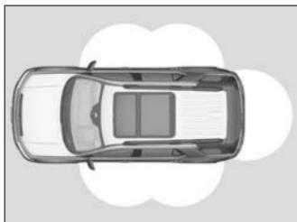
When you carry the keyless remote, you can lock/unlock the doors and fuel fill door, and open the tailgate.
