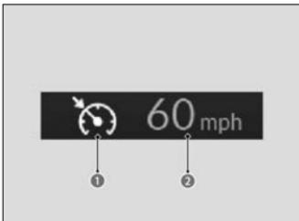
When driving at 20 mph (30 km/h) or above, press the **RES/+/SET/-** switch up or down.
