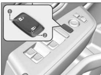
Press the master door lock switch in as shown to lock or unlock all doors, fuel fill door, and the tailgate.
