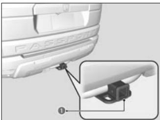
Your vehicle has a class 3 trailer hitch as standard equipment.
