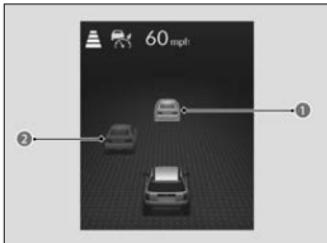
If a vehicle ahead enters the detectable range, icon (1) appears, and the system adjusts your vehicle's speed within the set range in order to keep the vehicle's set following-interval.
