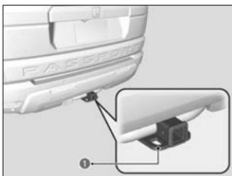
Trailer Hitch safety chain loops and receiver are rated for off-road recovery.
