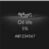
Oil life 5% AB1234567                                                                           | The remaining engine oil life is 5 to 1 percent. Roll the right selector wheel to switch to another display.                                                                                                                                                    |
