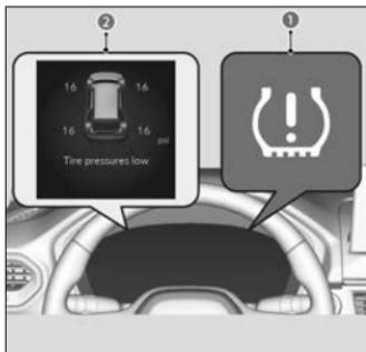
Monitors the tire pressure while you are driving. If your vehicle's tire pressure becomes significantly low, the Low Tire Pressure/TPMS indicator (1) comes on and the **Tire pressures low** message (2) appears.
