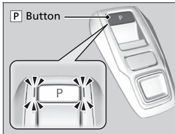
Park your vehicle in a safe place with the power mode in ON, then apply the brakes and press the P button to put the transmission in Park.
