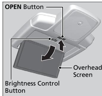
Push the **OPEN** button, then pull down the screen to the first or second detent until it latches.
