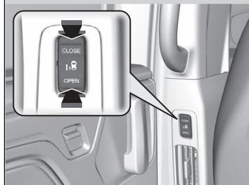
To resume the power sliding door operation, press the same switch again.
