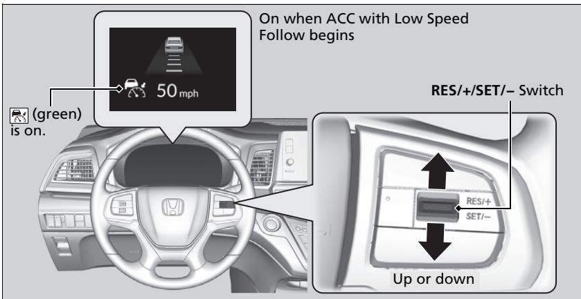
**When driving at about 25 mph (40 km/h) or above:** Take your foot off the pedal and press the **RES/+SET/-** switch up or down when you reach the desired speed. The moment you release the switch, the set speed is fixed, and ACC with Low Speed Follow begins.
