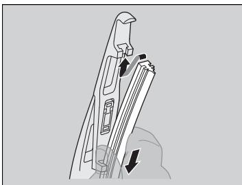
5. Slide the new wiper blade onto the holder.
