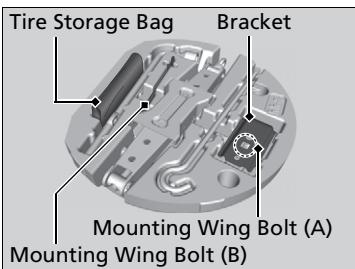
The tire storage bag, bracket, mounting wing bolt (A) and mounting wing bolt (B) are in the tool case.
