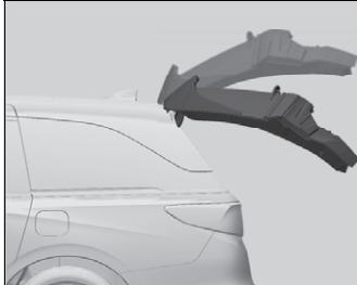
The extent to which the power tailgate automatically opens can be programmed.
