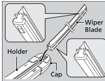
5. Insert the flat side of the new wiper blade onto the bottom part of the holder. Insert the blade all the way.
