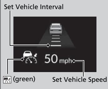
When ACC with Low Speed Follow starts operating, the vehicle icon, interval bars, and set speed appear on the gauge.
