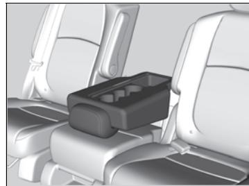
Pull up the strap and fold down the center backrest to use as an armrest.
