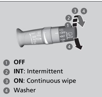
The rear wiper and washer can be used when the power mode is in ON.
