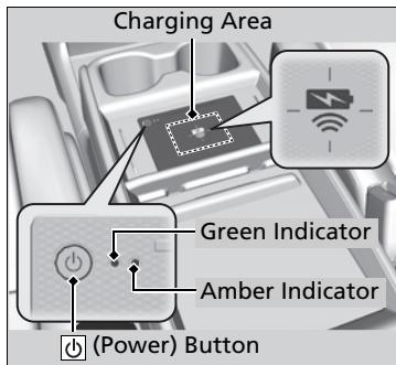
1. To turn the system on and off, press and hold the
