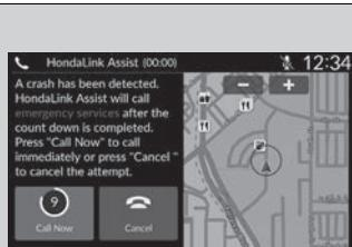
If your vehicle's airbags deploy or if the unit detects that the vehicle is severely impacted, your vehicle automatically will attempt to connect to the HondaLink operator. If connected, information about your vehicle, its location, and its condition can be sent to the operator\*<sup>1</sup>; you also can speak to the operator when connected.
