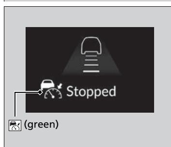
If no vehicle is ahead of you before you resume driving, depressing the accelerator pedal will resume operation of ACC with Low Speed Follow within the prior set speed.
