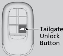
Press the tailgate unlock button to unlock the tailgate.
