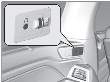
The headphone connector for the rear entertainment system is on the left side of the third row outer seats. The connector has its own volume control.
