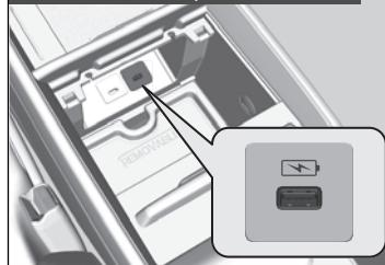
On the back of the console compartment (3.0A)
