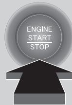
If you carry the keyless remote and press **ENGINE START/STOP** button without depressing the brake pedal, the power mode will change in this order: VEHICLE OFF→ACCESSORY→ON→VEHICLE OFF.
