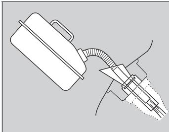
6. Fill the tank with fuel from the portable fuel container.
