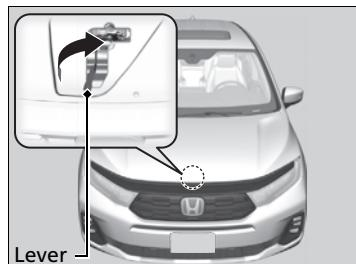
3. Pull up the hood latch lever (located under the front edge of the hood to the center) and raise the hood. Once you have raised the hood slightly, you can release the lever.
