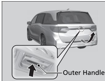
When all the doors are unlocked or press the tailgate unlock button\* on the remote transmitter, the tailgate is unlocked.
