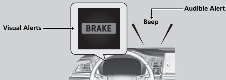
You can change the distance (**Long/Normal/Short**) between vehicles at which the system's earliest collision alert will come on.
