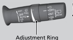
When you push the lever down to **AUTO**, the windshield wipers sweep once, and go into the automatic mode.
