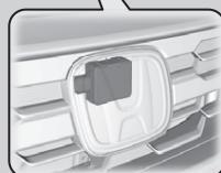
The radar sensor is inside the front grille.
