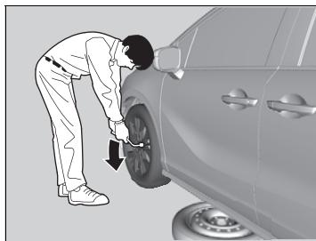
**8.** Loosen each wheel nut about one turn using the wheel nut wrench.
