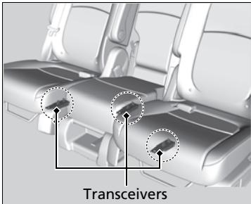
A transceiver is installed in second row removable seats to wirelessly communicate the seat belt fastening information to the vehicle. It will automatically connect to the vehicle whenever the seat is in or near its installation position.
