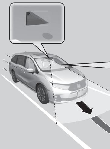
When you operate the turn signals to change lanes, the system is suspended, and resumes after the signals are off.
