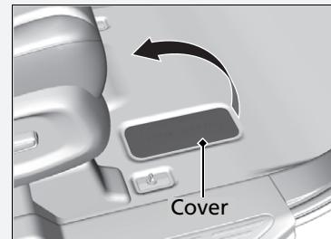
The interior vehicle identification number (VIN) is located under the cover.
