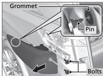
3. Use a Phillips-head screwdriver to remove the bolts.
