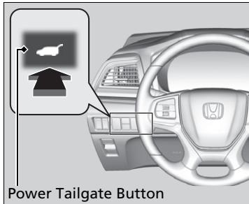
To open or close the power tailgate, press the power tailgate button for about one second.
