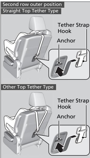
3. Raise the head restraint to its highest position, then route the tether strap outside/between the head restraint legs, and secure the tether strap hook to the anchor. Make sure the strap is not twisted.
