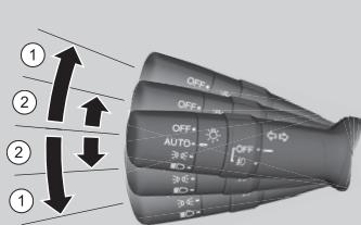
The turn signals can be used when the power mode is in ON.
