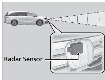
The radar sensor is behind the Honda emblem on the front grille.
