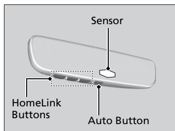
When you are driving after dark, the automatic dimming rearview mirror and power door mirrors\* reduces the glare from headlights behind you. Press the auto button to turn this function on and off. When activated, the auto indicator comes on.
