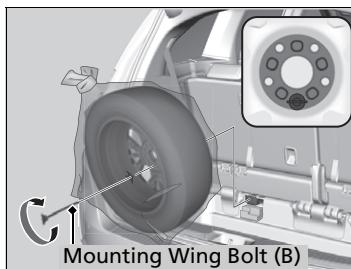
5. Install the flat tire on the bracket with the inside of the wheel facing toward you.
