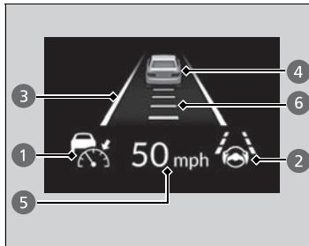
You can see the current state of Adaptive Cruise Control (ACC) with Low Speed Follow, Lane Keeping Assist System (LKAS).
