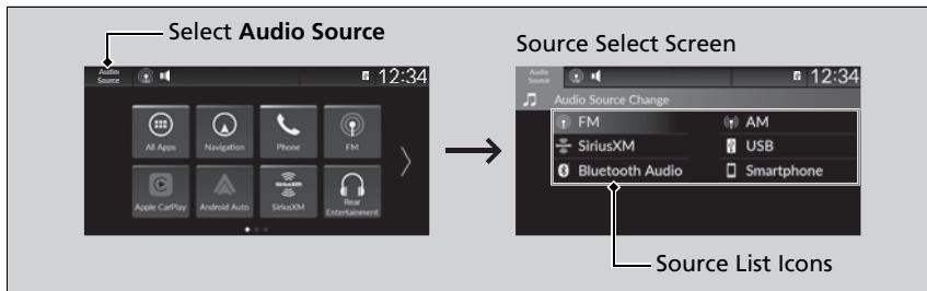
Select **Audio Source** in the header area, then select an icon on the source list to switch the audio source.
