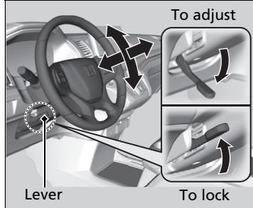
1. While the vehicle is stopped, push the steering wheel adjustment lever down.
