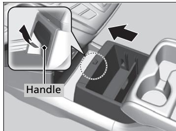
To open the console box, pull the handle and slide the box forward.
