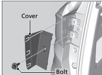
1. Use a Phillips-head screwdriver to remove the bolt.
