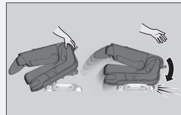
Raise the seat-back to an upright position, then rock the seat-back and forth to confirm both the inner and outer latches are securely locked into position.
