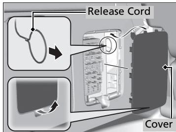
1. Open the tailgate and remove the cover on the left side of cargo area.
