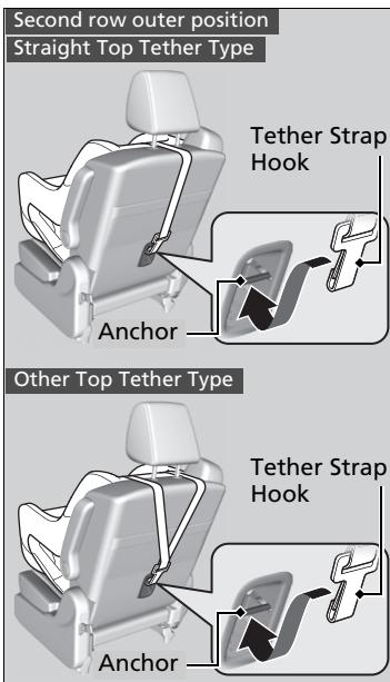
2. Raise the head restraint to its highest position, then route the tether strap outside/through the head restraint legs. Make sure the strap is not twisted.
