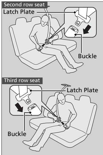
**3. Insert the latch plate into the buckle.**
