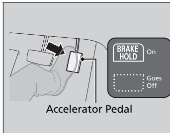
Depress the accelerator pedal while the transmission is in a position other than **P** or **N**. The system is canceled and the vehicle starts to move.
