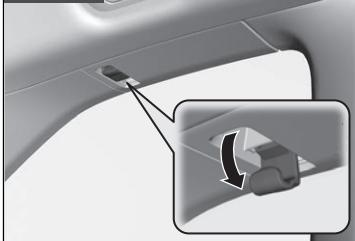
There are coat hooks under the grab handles in the second row, and under the window frames in the third row. Pull it down to use it.
