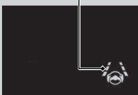
When the LKAS is suspended, green lines on the gauge disappear, and the beeper sounds (if activated).
