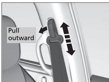
1. Move the anchor up and down while pulling the shoulder anchor outward.
