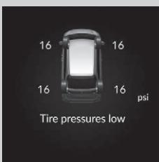
**Tire pressures low** is displayed when a tire has significantly low pressure. The specific tire is displayed on the screen.
