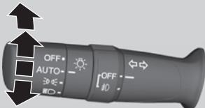
The lights will turn on automatically depending on the ambient brightness. They can also be switched on and off manually.
