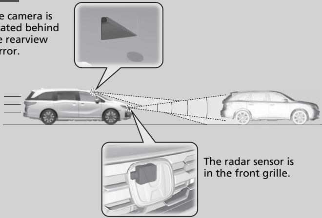
The system starts monitoring the roadway ahead when your vehicle speed is about 3 mph (5 km/h) or above and there is a vehicle in front of you.
