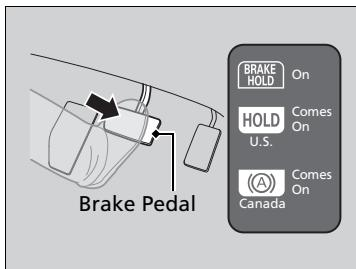
Depress the brake pedal to come to a complete stop. The transmission must not be in **P** or **R**.
