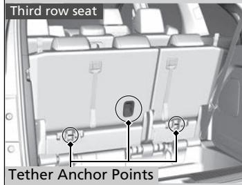
A tether anchor point is provided behind each second and third row seating position. If you have a child seat that comes with a tether but can be installed with a seat belt, the tether may be used for additional security.
