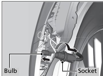
1. Turn the steering wheel all the way to the opposite side from the light being replaced.
