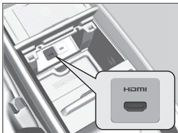
There is an HDMI™ port in the console compartment. The rear entertainment system will accept HDMI™ cable connections with video equipment that is equipped with an HDMI™ port.
