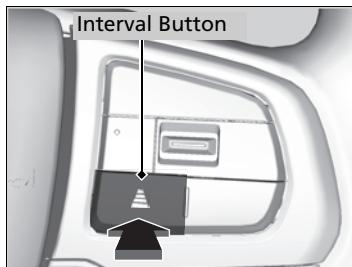
Press the interval button to change the ACC with Low Speed Follow following-interval. Each time you press the button, the following-interval (the interval behind a vehicle detected ahead of you) setting cycles through short, middle, long, and extra long following-intervals.
