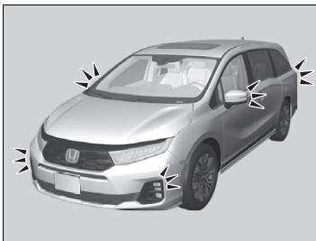
If the engine starts successfully, some exterior lights flash six times.
