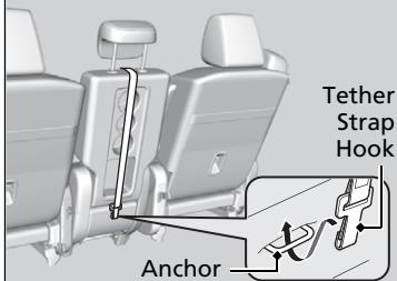
3. Secure the tether strap hook to the anchor.
