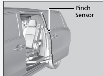
Do not touch the pinch sensor located at the front edge of the power sliding door. Do not damage the sensor. The power sliding door may not operate properly.
