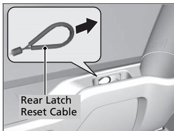
3. Pull the rear latch reset cable (yellow) towards the front of the vehicle until it bottoms out (about 9/16 inch [15 mm]).
