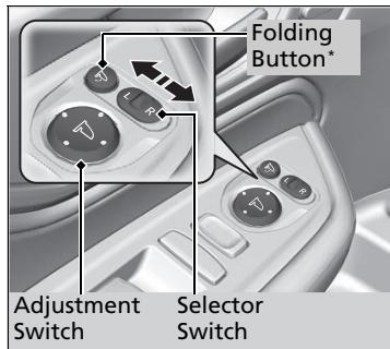
You can adjust the door mirrors when the power mode is in ON.
