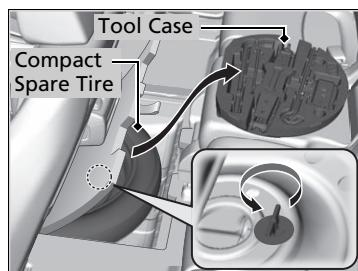
4. Take the tool case out of the compact spare tire well. Take the jack and wheel nut wrench out of the tool case.
