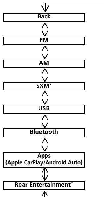
To use the audio system function, the power mode must be in ACCESSORY or ON.
