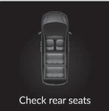
A reminder appears on the driver information interface and an alert will sound when the power mode is set to VEHICLE OFF.
