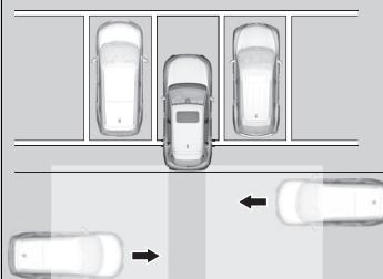
When a vehicle is detected approaching from a rear corner, Cross Traffic Monitor alerts you with a buzzer and a displayed warning.
