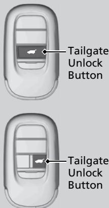
Press the tailgate unlock button to unlock the tailgate.
