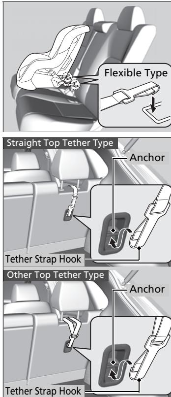
2. Raise the head restraint to its highest position, then route the tether strap between the head restraint legs, and secure the tether strap hook to the anchor. Make sure the strap is not twisted.
