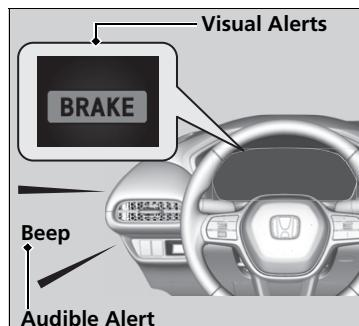
The system provides visual and audible alerts of a possible collision, and stops if the collision is avoided.
