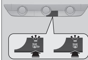
The rear defogger and heated door mirror\* automatically switch off after 10-30 minutes depending on the outside temperature.
