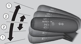
The turn signals can be used when the power mode is in ON.
