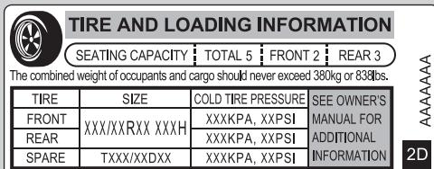
This figure includes the total weight of all occupants, cargo, and accessories, and the tongue load if you are towing a trailer.
