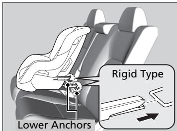
1. Place the child seat on the vehicle seat, then attach the child seat to the lower anchors according to the instructions that came with the child seat.
