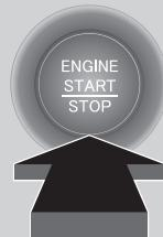
If you carry the keyless remote and press **ENGINE START/STOP** button without depressing the brake pedal, the power mode will change in this order: VEHICLE OFF→ACCESSORY→ON→VEHICLE OFF.
