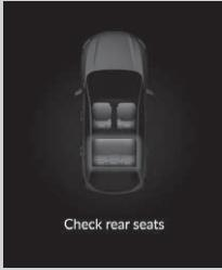
A reminder appears on the driver information interface and an alert will sound when the power mode is set to VEHICLE OFF.
