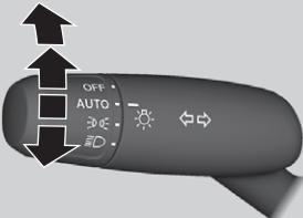
The lights will turn on automatically depending on the ambient brightness. They can also be switched on and off manually.
