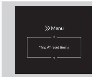
4. Roll the left selector wheel until "**Trip A**" **reset timing** appears on the display, then press the left selector wheel.
