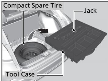
2. Take the tool case out of the cargo area. Take the wheel nut wrench, jack handle bar and jack out of the tool case.
