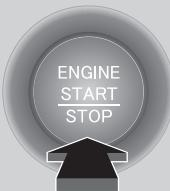
3. Press the **ENGINE START/STOP** button without depressing the accelerator pedal.
