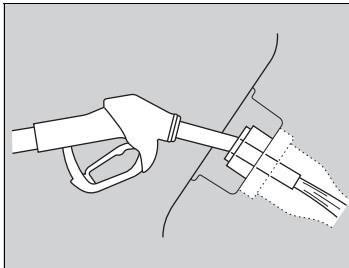
6. Place the end of the filler nozzle on the lower part of filler opening, then insert it slowly and fully.
