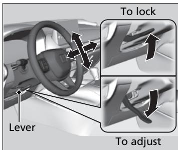
1. While the vehicle is stopped, push the steering wheel adjustment lever down.
