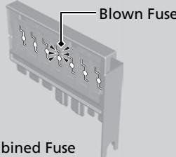
**5.** Inspect the small fuses in the engine compartment and the vehicle interior.
