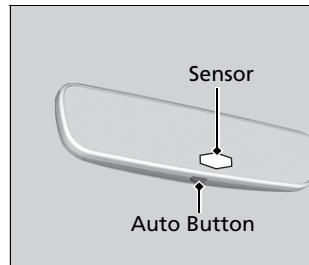
When you are driving after dark, the automatic dimming rearview mirror reduces the glare from headlights behind you. Press the AUTO button to turn this function on and off. When activated, the AUTO indicator comes on.
