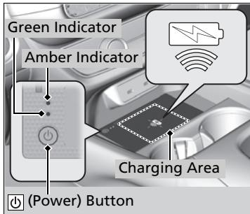
1. To turn the system on and off, press and hold the
