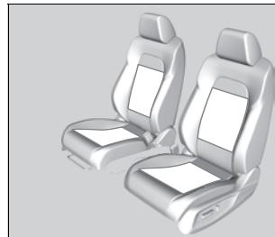
The seat heaters can be used when the power mode is in ON.
