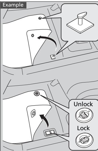
The driver's floor mat hooks over the floor anchors, which keep the mat from sliding forward.
