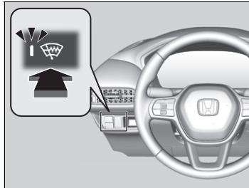
Press the heated windshield button to deice the windshield at the wiper park area of the windshield when the power mode is in ON.
