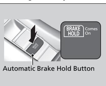
Fasten your seat belt properly, then start the engine. Press the automatic brake hold button.
