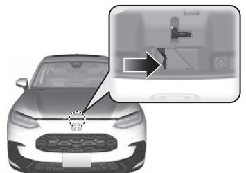
3 When finished, close the hood and make sure it is firmly locked in place.
