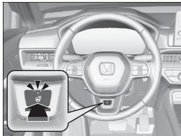
The heated steering wheel can be used when the power mode is in ON.
