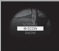
Facilitates fuel-efficient driving.
