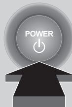
If you carry the keyless remote and press the **POWER** button without depressing the brake pedal, the power mode will change in this order: VEHICLE OFF→ACCESSORY→ON→VEHICLE OFF.
