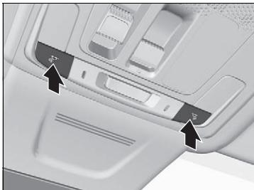
The map lights can be turned on and off by pressing the switches.
