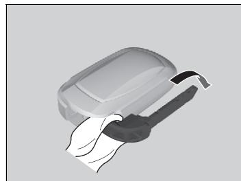
2. With the buttons facing down, remove the upper half of the cover by carefully prying on the slot with the key grip.
