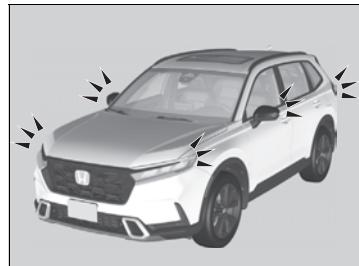
If the power system is turned on successfully, some exterior lights flash six times.
