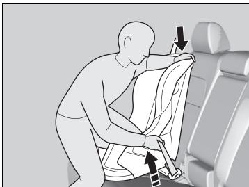
5. Grab the shoulder part of the seat belt near the buckle, and pull up to remove any slack from the lap part of the belt.
