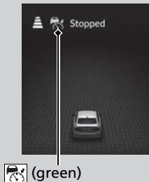
If no vehicle is ahead of you before you resume driving, depress the accelerator pedal and ACC with Low Speed Follow will operate again within the prior set speed.
