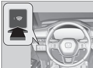
Press the heated windshield button to deice the windshield at the wiper park area and along the driver side edge of the windshield when the power mode is in ON.
