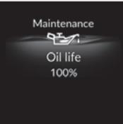
*2 | When you select the Maintenance Minder screen, it displays codes for maintenance items due at the next engine oil change, along with the percentage of engine oil life remaining.                                                                                                                                                                   | -                                                                                                                                  |
