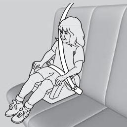
If a lap/shoulder seat belt cannot be used properly, position the child in a booster seat in the rear seat. For the child's safety, check that the child meets the booster seat manufacturer's recommendations.
