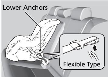
4. Attach the child seat to the lower anchors according to the instructions that came with the child seat.
