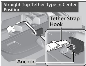
3. Secure the tether strap hook to the anchor.
