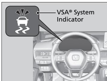
When VSA® activates, you may notice that the engine and motor do not respond to the accelerator. You may also notice some noise from the hydraulic brake system. You will also see the indicator blink.
