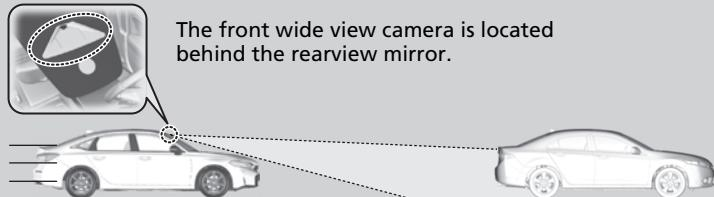
The system starts monitoring the roadway ahead when your vehicle speed is about 3 mph (5 km/h) or above and will search for a vehicle (including motorcycles), pedestrian, or moving bicycle in front of you.
