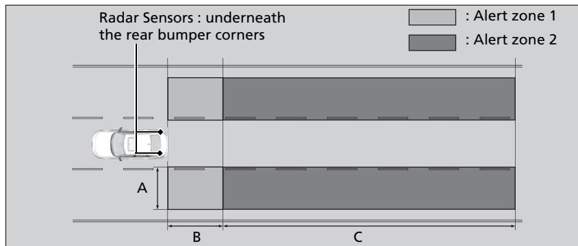
The initially set alert zone is alert zone 1. Over time, after the vehicle has been driven on straight roads with traffic and roadside objects, the system will adapt and expand the alert zone (alert zone 1 and 2).
