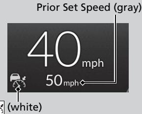
The set speed cannot be set or resumed when ACC with Low Speed Follow has been turned off using the button. Press the button to activate the system, then set the desired speed.
