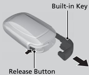
The built-in key can be used to unlock the doors when the keyless remote battery becomes weak and the power door unlock operation is disabled.
