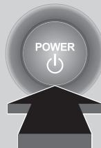
If you carry the keyless remote and press **POWER** button without depressing the brake pedal, the power mode will change in this order: VEHICLE OFF → ACCESSORY → ON → VEHICLE OFF.
