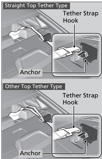
5. Open the tether anchor cover behind the head restraint.
