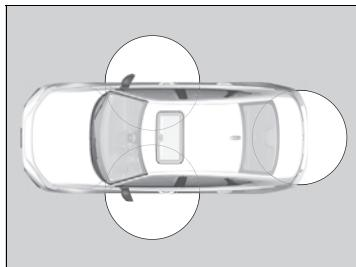
When you carry the keyless remote, you can lock/unlock the doors and fuel fill door, and open the trunk.
