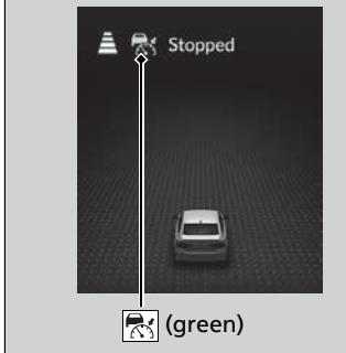
If no vehicle is ahead of you before you resume driving, depress the accelerator pedal and ACC with Low Speed Follow will operate again within the prior set speed.
