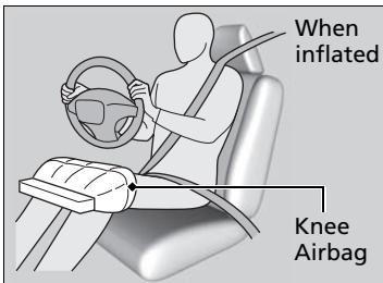
The driver's and front passenger's knee airbag deploy at the same time as the driver's and front passenger's airbag respectively.
