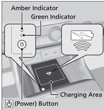
1. To turn the system on and off, press and hold the
