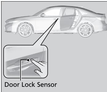
The vehicle will automatically lock after you lock the doors in advance then close the doors.
