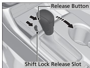
5. Insert the key into the shift lock release slot.
