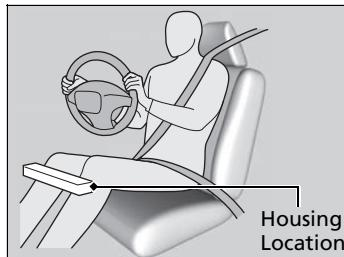
The knee airbag for the driver and the one for the front passenger are housed under the steering column and the glove box respectively.
