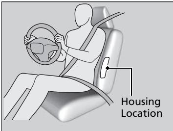
The side airbags are housed in the outside edge of the driver's and passenger's seat-backs and next to the outer rear seating positions.
