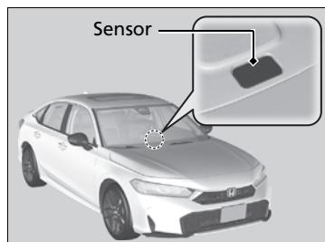
The automatic climate control system is equipped with sensors. Do not cover or spill any liquid on them.
