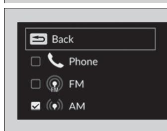
3. Roll the left selector wheel to scroll between audio sources, then press the left selector wheel to check or uncheck them.
