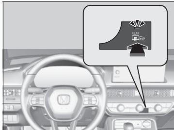
The rear defogger and heated door mirror automatically switches off after 10-30 minutes depending on the outside temperature. However, if the outside temperature is 32°F (0°C) or below, it does not automatically switch off.
