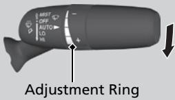
When you push the lever down to **AUTO**, the windshield wipers sweep once, and go into the automatic mode.
