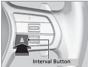
Press the Interval button to change the ACC with Low Speed Follow following-interval. Each time you press the button, the following-interval (the interval behind a vehicle detected ahead of you) setting cycles through furthest, far, mid, and nearest following-intervals.
