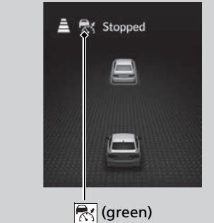
Your vehicle also stops automatically. The **Stopped** message appears on the gauge. When the vehicle ahead of you starts again, if you press the **RES/+/SET/-** switch up or down, or depress the accelerator pedal, ACC with Low Speed Follow will operate again within the previously set speed.
