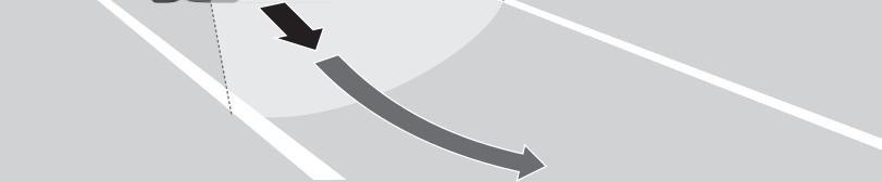
When you operate the turn signals to change lanes, the system is suspended, and resumes after the signals are off.
