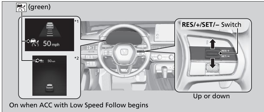
**When driving at about 20 mph (30 km/h) or above:** Take your foot off the pedal and press the **RES/+SET/-** switch up or down when you reach the desired speed. The moment you release the switch, the set speed is fixed, and ACC with Low Speed Follow begins.
