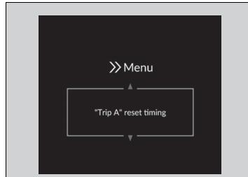
4. Roll the left selector wheel until "**Trip A**" **reset timing** appears on the display, then press the left selector wheel.
