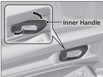
Unlocking and opening the driver's door from the inner handle unlocks all the other doors.
