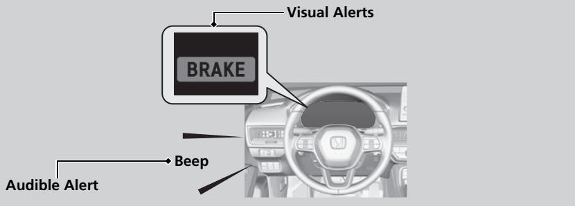
You can change the distance (**Long/Normal/Short**) between vehicles at which the system's earliest collision alert will come on.
