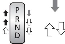
Depress the brake pedal and press the shift lever release button to shift.
