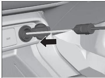
7. Plug in the air compressor to the accessory power socket.
