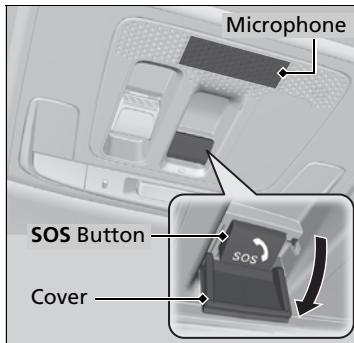
If you need to make an emergency call, you can establish a connection manually. Press the **SOS** button and hold it for more than 0.5 seconds.
