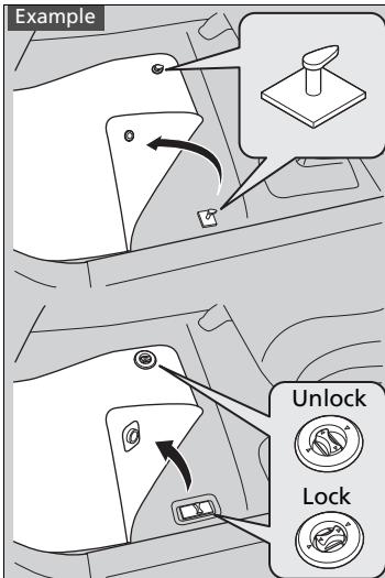
The driver's floor mat hooks over floor anchors, which keep the mat from sliding forward.
