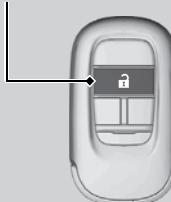
Press the unlock button, and then within 10 seconds, press it again and hold it.
