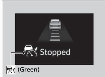
Your vehicle also stops automatically. The **Stopped** message appears on the gauge. When the vehicle ahead of you starts again, if you press the **RES/+ / SET / -** switch up or down, or depress the accelerator pedal, ACC with Low Speed Follow will operate again within the previously set speed.
