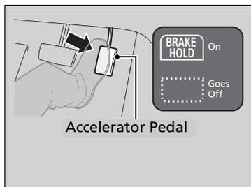
Depress the accelerator pedal while the transmission is in a position other than **P** or **N**. The system is canceled and the vehicle starts to move.
