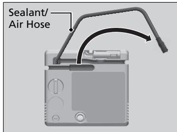
2. Remove the sealant/air hose from the packaging.
