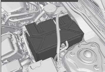
The condition of the battery is monitored by a sensor located on the negative terminal of the battery. If there is a problem with this sensor, the driver information interface will display a warning message. If this happens, have your vehicle inspected by a dealer.
