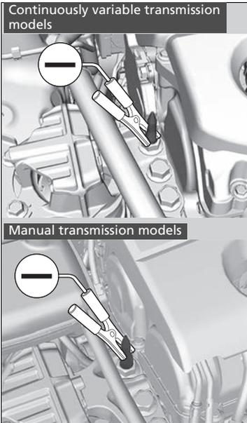
5. Connect the other end of the second jumper cable to the stud bolt as shown. Do not connect this jumper cable to any other part.
