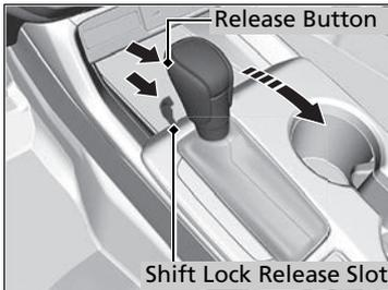
5. Insert the key into the shift lock release slot.
