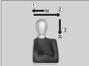
1. Depress the clutch pedal, move the shift lever all the way to the left, and shift to **R**.
