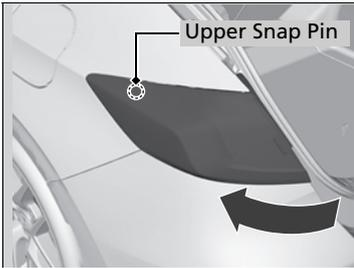
**4.** Rotate the taillight outward to release the upper snap pin.
