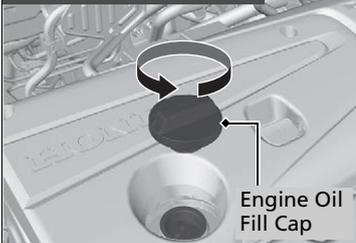
1. Unscrew and remove the engine oil fill cap.
