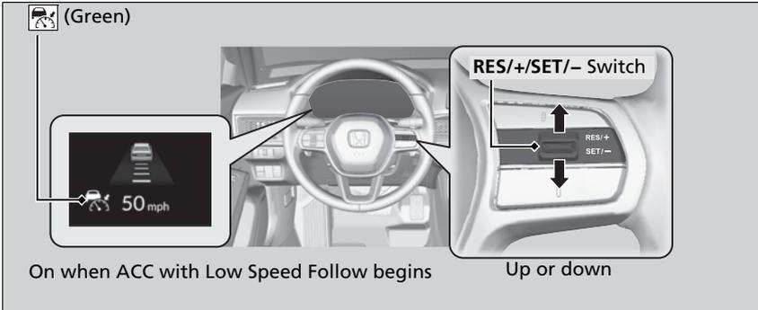
**When driving at about 20 mph (30 km/h) or above:** Take your foot off the pedal and press the **RES/+ / SET/-** switch up or down when you reach the desired speed. The moment you release the switch, the set speed is fixed, and ACC with Low Speed Follow begins.
