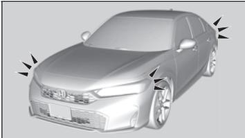
If the engine starts successfully, some exterior lights flash six times.
