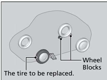
5. Place a wheel block or rock in front and rear of the wheel diagonal to the flat tire.
