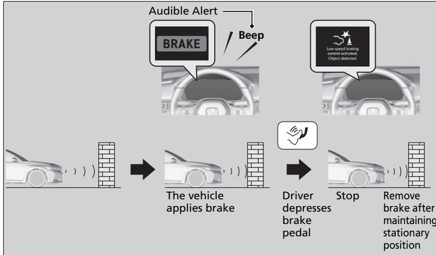
If only the rear sensors are turned off using the parking sensor system, the Low Speed Braking Control will not work when reversing.
