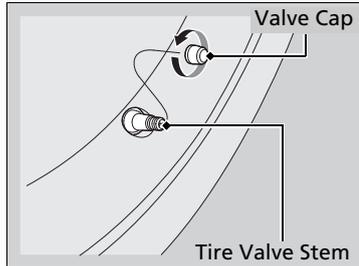
1. Remove the valve cap from the tire valve stem.
