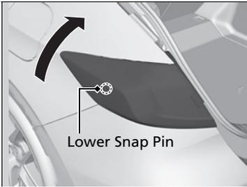
**3.** Grasp underneath the taillight and rotate it upward to release the lower snap pin.
