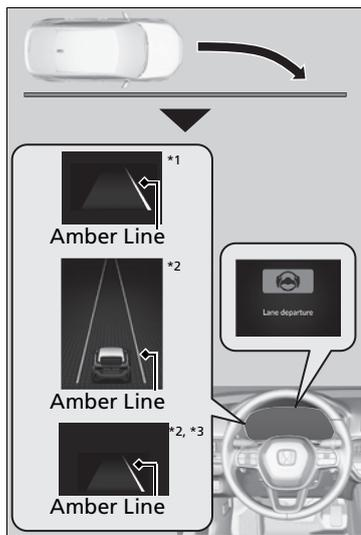
The front wide view camera behind the rearview mirror monitors left and right lane markings in white or yellow, the outer edge of the pavement (into grass or gravel road shoulder) or a detected oncoming vehicle. If your vehicle approaches any detected lane markings, the outer edge of the pavement (into grass or gravel road shoulder) or a detected oncoming vehicle when the turn signals have not been engaged, the system activates.
