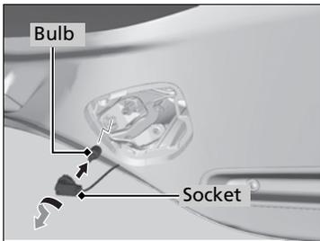
2. Turn the socket counter-clockwise and remove it.
