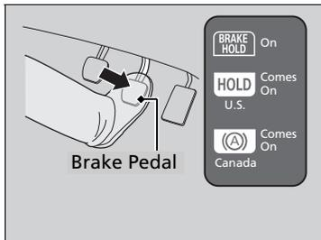
Depress the brake pedal to come to a complete stop.
