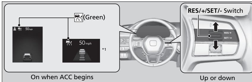
Take your foot off the pedal and press the **RES/+SET/-** switch up or down when you reach the desired speed. The moment you release the button, the set speed is fixed, and ACC begins.
