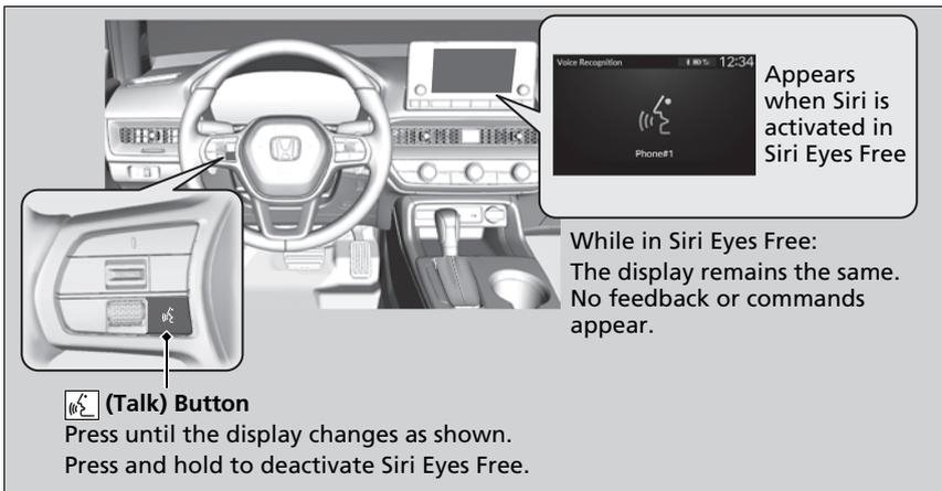
The diagram shows a car's interior with a steering wheel and a central display. A callout box shows the display when Siri is activated, displaying "Voice Recognition" and "Phone1". Another callout box shows the Siri Talk button on the steering wheel. A third callout box explains that while in Siri Eyes Free mode, the display remains the same and no feedback or commands appear.
