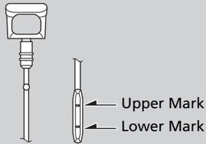
4. Remove the dipstick again, and check the level. It should be between the upper and lower marks. Add oil if necessary.
