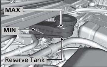
The fluid level should be between the **MIN** and **MAX** marks on the side of the reserve tank.
