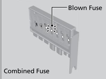
5. Inspect the small fuses in the engine compartment and the vehicle interior.
