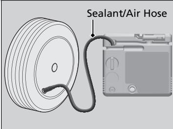
4. Recheck the air pressure using the sealant/air hose on the compressor.
