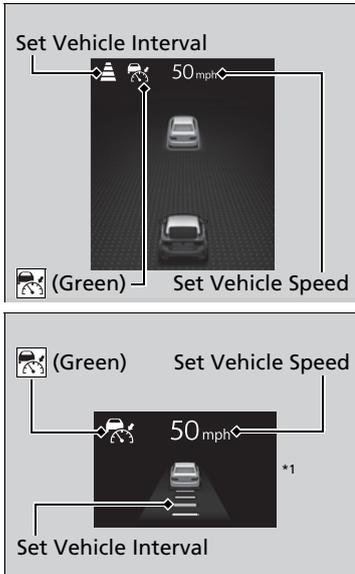
When ACC starts operating, the vehicle icon, distance bars and set speed appear on the gauge.
