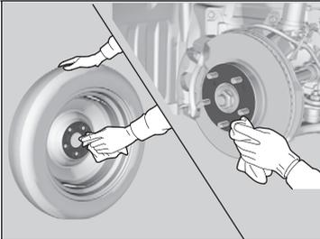
2. Wipe the mounting surfaces of the wheel with a clean cloth.
