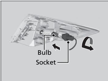
**6.** Turn the socket counter-clockwise and remove it.
