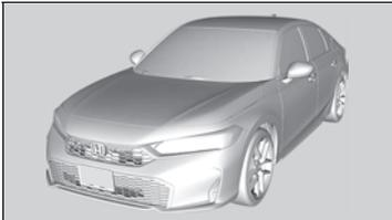
When the remote is out of the keyless access system range, the exterior lights will not flash. The engine will not stop.
