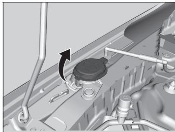
If the level is low, fill the washer reservoir.
