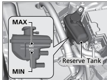
1. Check the coolant level in the tank.
