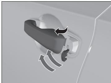
If the unlock button of the keyless remote does not work, use the built-in key instead. The keyhole is behind the door handle.
