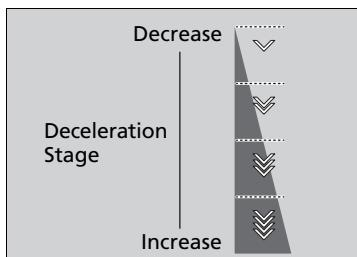
The default deceleration stage is . Each paddle selector operation makes a single stage deceleration change.
