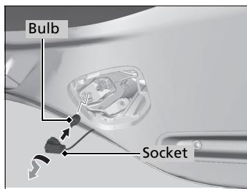
2. Turn the socket counter-clockwise and remove it.
