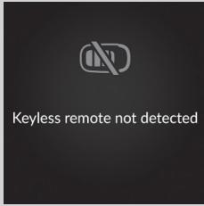
When the power mode is set to any mode other than OFF and you remove the keyless remote from the vehicle and shut the door, an alarm will sound. If the alarm continues to sound, place the keyless remote in another location.
