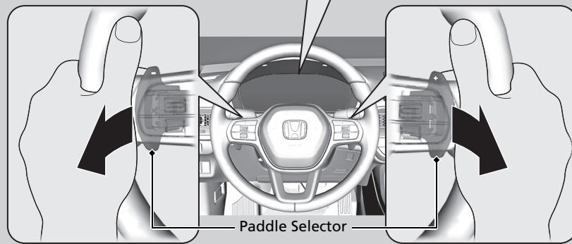
Increase the deceleration stage when pulling the **-** paddle selector (left side)Decrease the deceleration stage when pulling the **+** paddle selector (right side)
