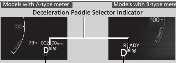
Shift Position Indicator (Transmission System Indicator)
