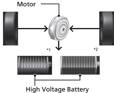
When decelerating without the accelerator being depressed or the brake pedal being applied, or while driving downhill, the electric motor acts as a generator that recovers a portion of the electrical energy that was used to accelerate the vehicle. This regenerative braking slows the vehicle in a manner similar to engine braking in a gasoline-powered vehicle. You can control the rate of deceleration by using the deceleration paddle selector.
