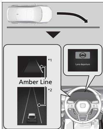
The front wide view camera behind the rearview mirror monitors left and right lane markings in white or yellow, the outer edge of the pavement (into grass or gravel road shoulder) or a detected oncoming vehicle. If your vehicle approaches any detected lane markings, the outer edge of the pavement (into grass or gravel road shoulder) or a detected oncoming vehicle when the turn signals have not been engaged, the system activates.
