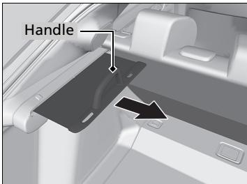
The cargo area cover can be used to cover the cargo space.
