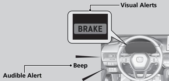
You can change the distance (**Long/Normal/Short**) between vehicles at which the system's earliest collision alert will come on.
