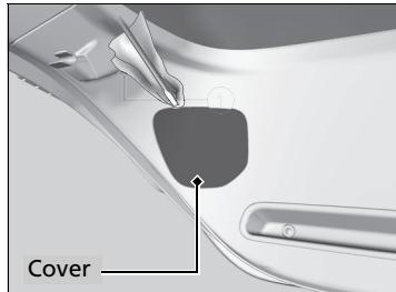
1. Remove the cover by prying on the edge using a flat-tip screwdriver.
