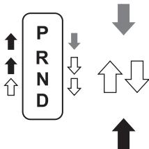
Depress the brake pedal and press the shift lever release button to shift.
