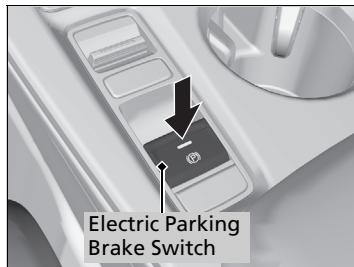
Manually releasing the parking brake using the switch helps your vehicle start slowly and smoothly when facing downhill on steep hills.
