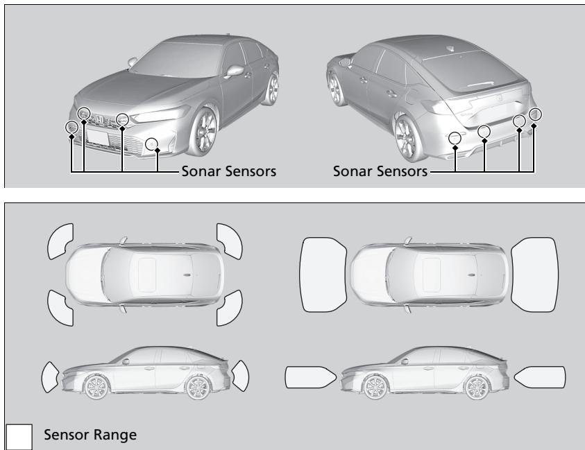
The sonar sensors are situated in the front and rear bumpers, and the front grille.
