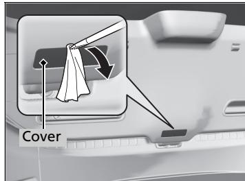
1. Use a flat-tip screwdriver and remove the cover on the back of the hatch.
