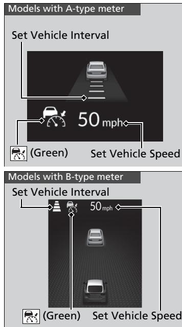
**When driving slower than about 20 mph (30 km/h):** If the vehicle is moving and the brake pedal is not depressed, pressing the switch fixes the set speed to about 20 mph (30 km/h) regardless of current vehicle speed. If your vehicle is stationary, you can set the vehicle speed even with the brake pedal depressed.
