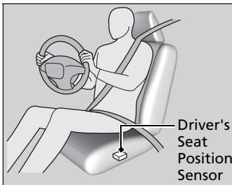
The driver's advanced airbag system includes a seat position sensor.
