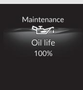
*2         | When you select the Maintenance Minder screen, it displays codes for maintenance items due at the next engine oil change, along with the percentage of engine oil life remaining.                                                                                                                                                                   | —                                                                                                                           |
