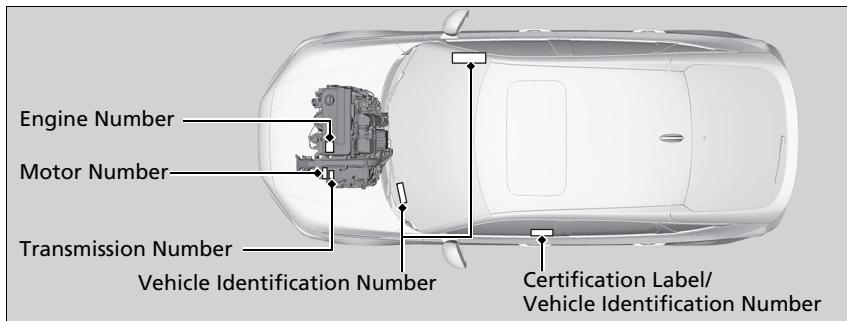
Vehicle Identification Number (VIN), Engine Number, Motor Number, and Transmission Number
