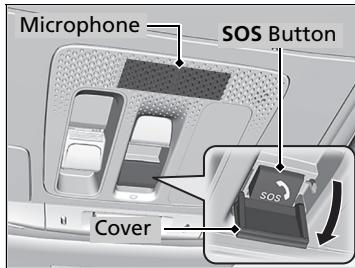
If you need to make an emergency call, you can establish a connection manually. Press the **SOS** button and hold it for more than 0.5 seconds.
