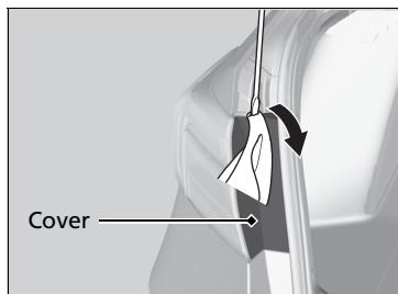
1. Pry on the edge of the cover using a flat-tip screwdriver to remove the cover.
