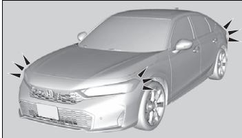
If the power system is turned on successfully, some exterior lights flash six times.
