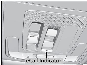
If your vehicle is involved in a collision, the vehicle will attempt to connect to an operator. Once a connection is established, your location information will be sent to an operator with whom you will be able to speak.
