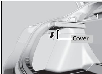
1. Open the hatch and remove the cover on the left side of cargo area.
