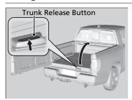
Push up the trunk release button on the trunk lid after all the doors are unlocked.
