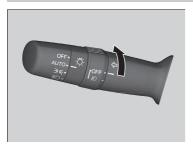
When the headlights are on, turn the fog light switch on to use the fog lights.
