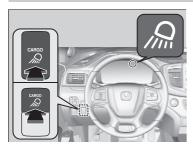
The bed lights can be turned on or off by pressing the button when the transmission is in  $\boxed{\mathbf{P}}$ .
