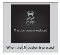
This button is on the driver side control panel. To partially disable VSA® functionality/ features, press and hold it until you hear a beep.
