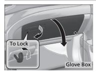
Pull the lever to open the glove box. You can lock the glove box with the built-in key.
