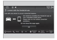
You can see the connection guide screen after launching HondaLink® when there is no connection to a network. If you do not need this guide, select check-box and select **OK**.
