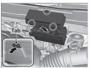
Fuse locations are shown on the fuse box cover. Locate the fuse in question by the fuse number and box cover number.
