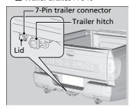
Open the lid of the socket (located next to the trailer hitch) to expose the 7-pin trailer connector.
