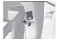
Locate the hood latch lever, push it to the side, and then raise the hood. Once you have raised the hood slightly, you can release the lever.
