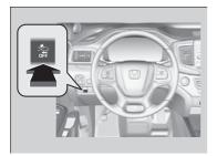
Press and hold the button until the beeper sounds to switch the system on or off.
