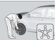
**5.** Lower the vehicle and remove the jack. Tighten the wheel nuts in the order indicated in the image. Go around tightening the nuts two to three times in this order.
