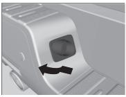
**1.** Remove the license plate light assembly by pulling it towards you, and then pulling the front edge upward.
