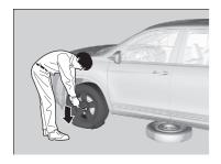
**8.** Loosen each wheel nut about one turn using the wheel nut wrench.
