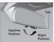
Flip the tab to switch the position.
