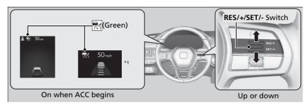
Take your foot off the pedal and press the **RES/+/SET/-** switch up or down when you reach the desired speed. The moment you release the button, the set speed is fixed, and ACC begins.
