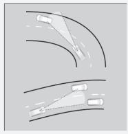
When the vehicle ahead of you moves away, such as when entering an interchange or rest area, ACC may continue to maintain the set following-interval for a short time.
