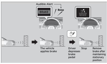
If only the rear sensors are turned off using the parking sensor system, the Low Speed Braking Control will not work when reversing.
