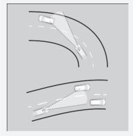
When the vehicle ahead of you moves away, such as when entering an interchange or rest area, ACC with Low Speed Follow may continue to maintain the set following-interval for a short time.
