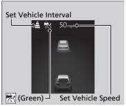
When ACC starts operating, the vehicle icon, distance bars and set speed appear on the gauge.
