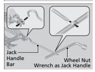
**3.** Raise the vehicle, using the jack handle bar and the jack handle, until the tire is off the ground.
