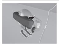
If the unlock button of the keyless remote does not work, use the built-in key instead. The keyhole is behind the door handle.
