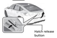
Press the hatch release button to unlock and open the hatch when you carry the keyless remote.
