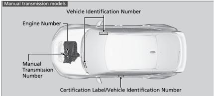
■ Vehicle Identification Number (VIN), Engine Number, and Transmission Number
