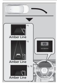
The front wide view camera behind the rearview mirror monitors left and right lane markings in white or yellow, the outer edge of the pavement (into grass or gravel road shoulder) or a detected oncoming vehicle. If your vehicle approaches any detected lane markings, the outer edge of the pavement (into grass or gravel road shoulder) or a detected oncoming vehicle when the turn signals have not been engaged, the system activates.
