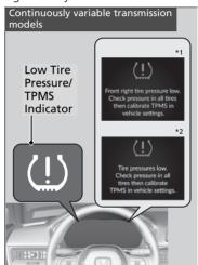
This will cause the low tire pressure/TPMS indicator to come on and a message to appear on the gauge.
