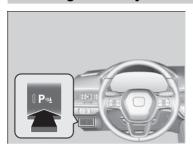
With the power mode in ON, press the parking sensor system button to turn on or off the system. The indicator in the button comes on when the system is on.
