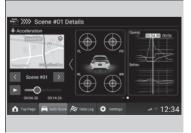
You can enlarge the graph by selecting it. After it has been enlarged, you can adjust the scale. The vertical axis is adjusted by pinching in or out on the screen, and the horizontal axis is adjusted by selecting the icons.
